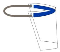
Face shield assembly is typically bonding polycarbonate or polyester (PET) film to a foam.
